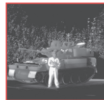
Range for Johnson's criteria, target deltaT = 2K, perfect atmospheric and optics transmissions, theoretical square pixel.
