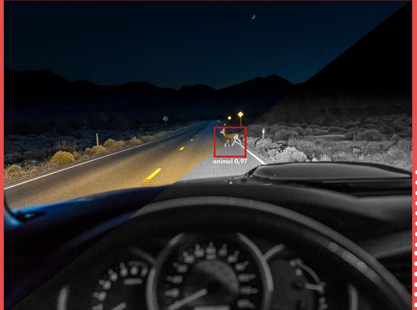
Thermal imaging application in emergency braking systems to prevent collision with obstacles, pedestrians, cyclists or animals, especially at night or in poor weather conditions
