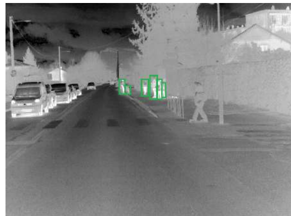
Same obstacle not detected as a pedestrian, thanks to thermal imaging system
