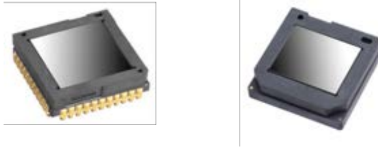
Figure 1.1. ATTO640D-04W (Left) versus YOCTO1024 (Right) Packages
