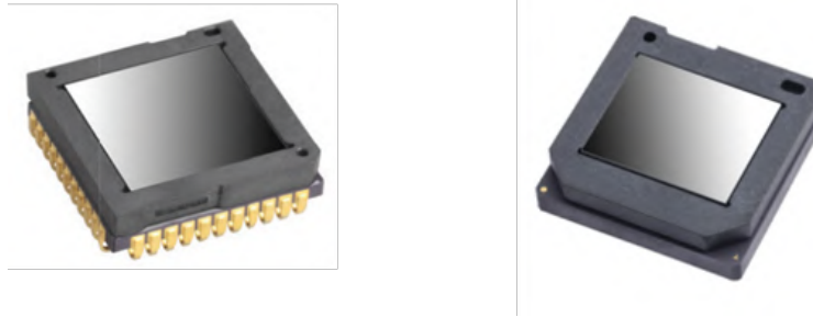
Figure 1.1. ATTO640D-04W (Left) versus YOCTO1024 (Right) Packages
