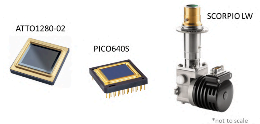
Figure 1.2. Uncooled (ATTO1280 & PICO640S) and cooled (SCORPIO LW) image sensors
